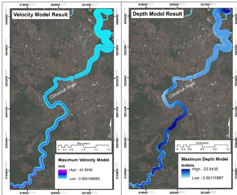
Figure 3. Flood inundation model results - velocity model (left) and depth model (right)
