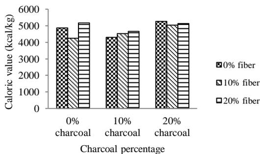
Figure 7. The effect of the percentage of palm shell, palm shell charcoal, and palm fibers to the caloric value of biopellet
