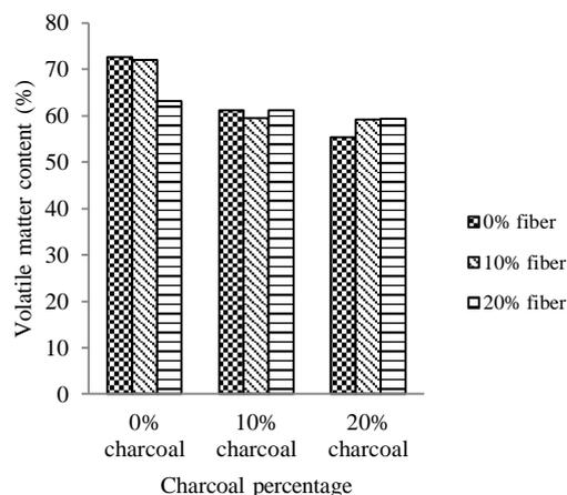
Figure 5. The effect of the percentage of palm shell, palm shell charcoal, and palm fibers to the volatile matter of biopellet
