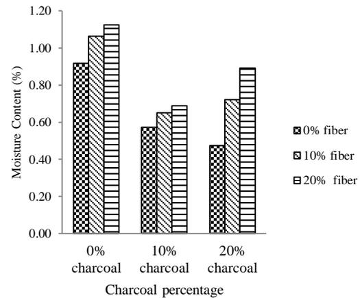
Figure 3. The effect of the percentage of palm shell, palm shell charcoal, and palm fibers to the moisture content of biopellet
