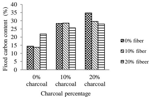
Figure 6. The effect of the percentage of palm shell, palm shell charcoal, and palm fibers to the fixed carbon of biopellet
