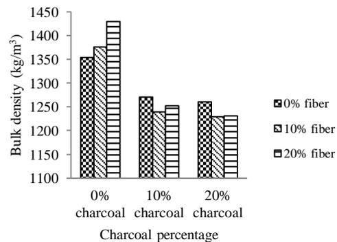
Figure 8. The effect of the percentage of palm shell, palm shell charcoal, and palm fibers to the bulk density of biopellet
