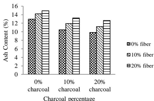
Figure 4. The effect of the percentage of palm shell, palm shell charcoal, and palm fibers to the ash content of biopellet
