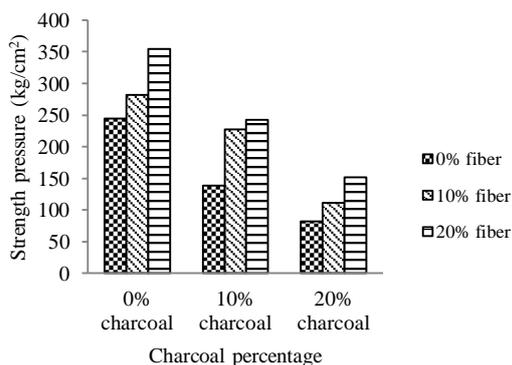
Figure 9. The effect of the percentage of palm shell, palm shell charcoal, and palm fibers to the strength pressure of biopellet
