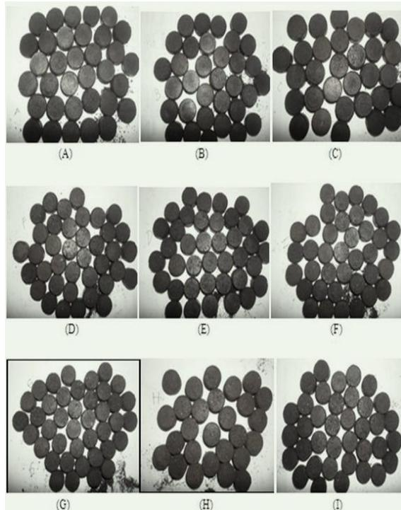
Figure 2. Biopellet of palm shell with the formulation palm shell: palm shell charcoal: palm fiber (A) 100:0:0 (B) 90:0:10; (C) 80:0:20; (D) 90:10:0; (E) 80:10:10 (F) 70:10:20; (G) 80:20:0; (H) 70:20:10; (I) 60:20:20
